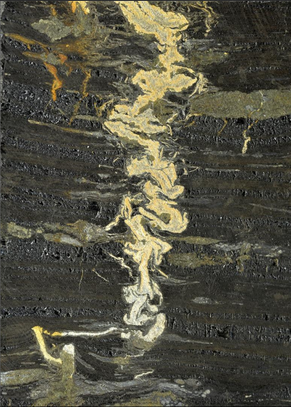
Highly crenulated pyrite cross-cutting alternating layers of dull and bright coal, the coal having semi-parallel layers and flattened concretions of mixed, dull pyrite/siderite. Bruce Cairncross photo ©.
