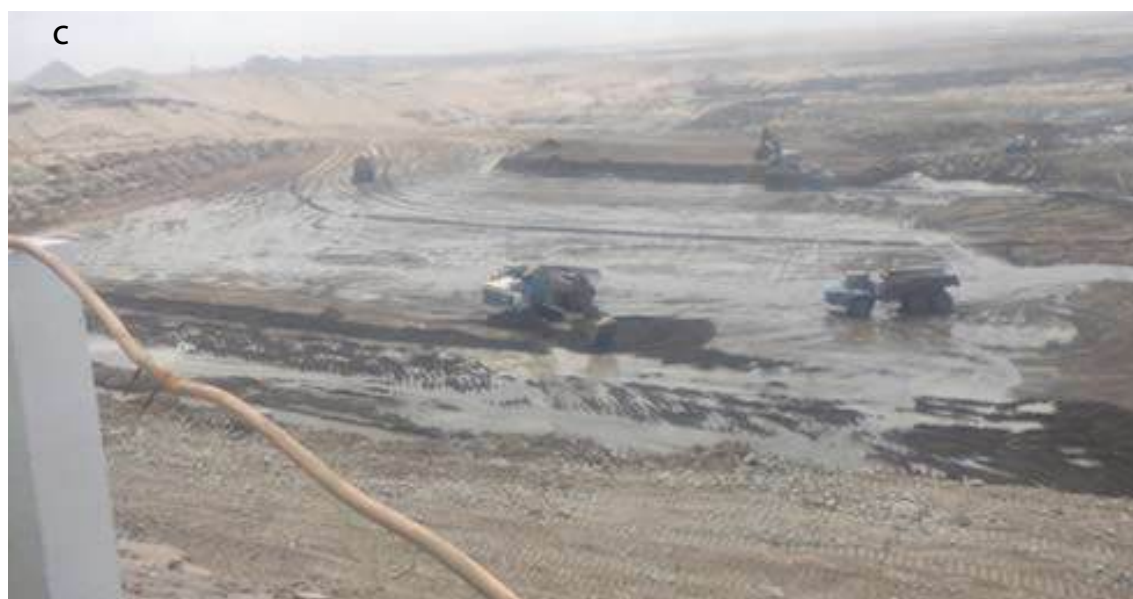
Namdeb. a) Bedrock cleaning (seawall in the background). b) Bedrock cleaning with Transvac. c) Overburden removal (view from on top of the seawall).
