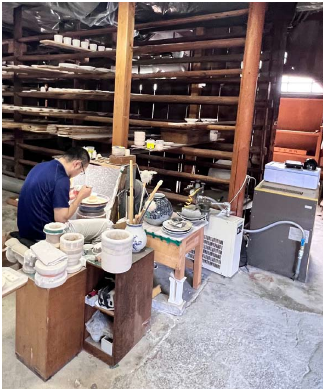
Potter at work in Imaemura pottery works, Arita. Note the electric kiln on the right for final firing of overglazed Iro Nabeshima porcelain.
