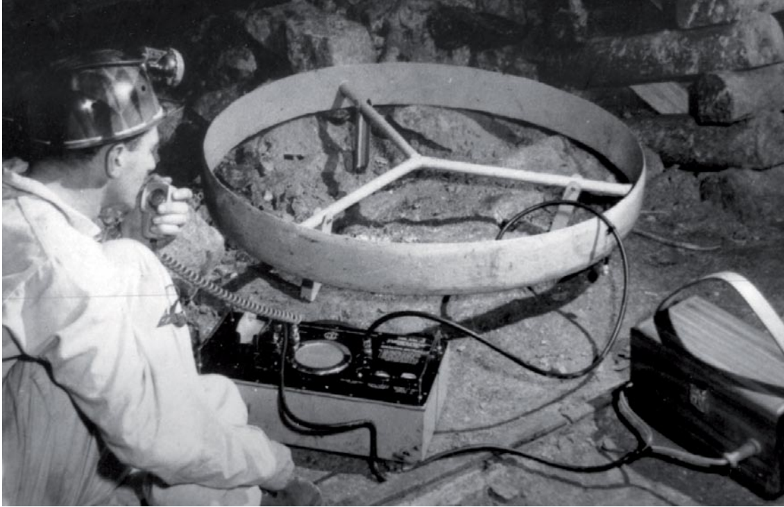
Fresh-air base set and large loop antenna.
